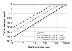
Figure 2. Illuminance vs. Output Voltage
