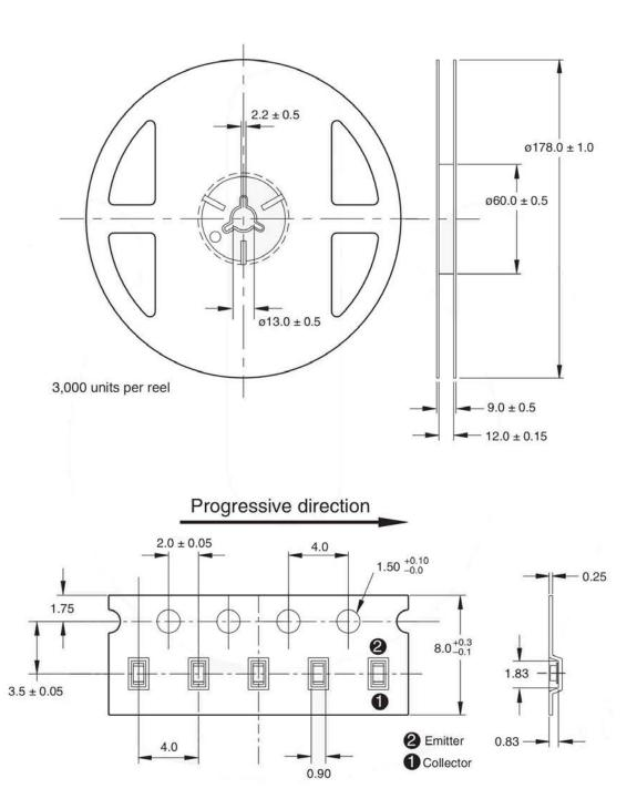
Note: Tolerances are ±0.1mm unless otherwise stated. All dimensions in mm.
