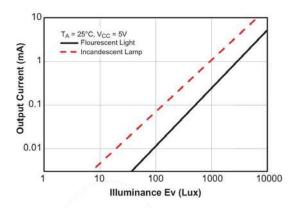
Figure 1. Illuminance vs. Output Photo Current
