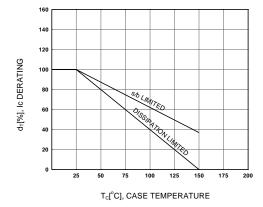
Figure 5. Derating Curve of Safe Operating Areas
