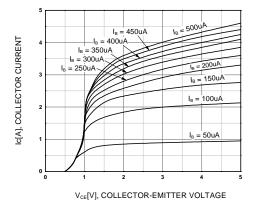
Figure 1. Static Characteristic
