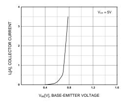
Figure 4. Base-Emitter On Voltage
