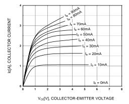
Figure 1. Static Characteristic
