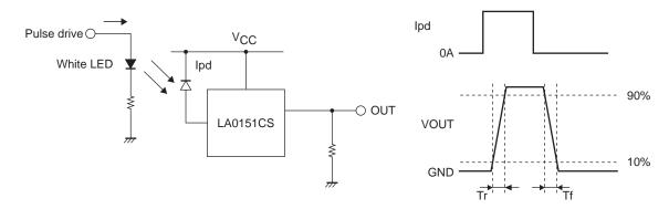
9. Reference value : min = 2.6V and typ = 2.8V when  $V_{\mbox{CC}}$  = 2.9V
