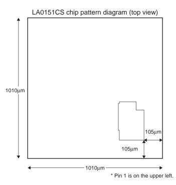
LA0151CS photo-receiving pattern enlarged diagram (effective area)
