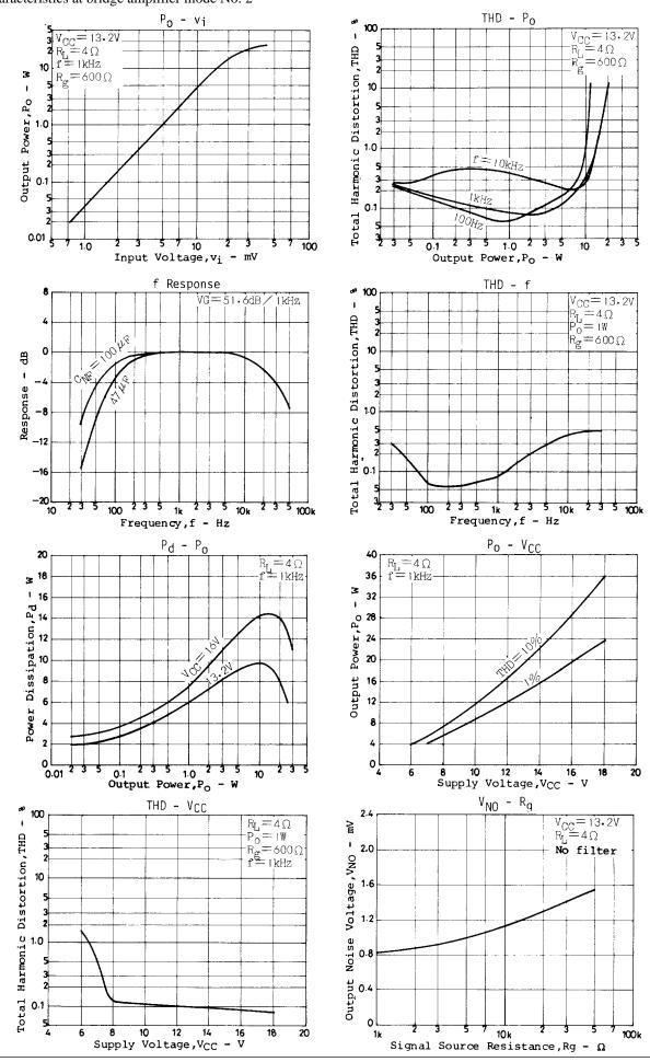
Characteristics at bridge amplifier mode No. 2
