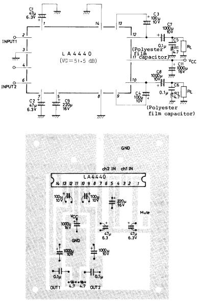
Sample printed circuit pattern for dual mode (Cu-foiled area) 60 x 70 mm<sup>2</sup>
