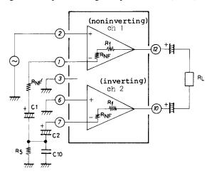
$$\begin{array}{l} R_{NF} = 50\Omega \; (typ), \; R_{f} = 20k\Omega \; (typ) \\ At \; R_{NF}' = 0 \; (recommended \; VG) \end{array}$$
