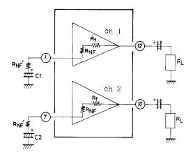
Voltage Gain Adjust at Bridge Amplifier Mode (No. 1)
