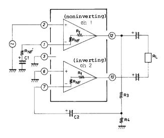
Voltage Gain Adjust at Bridge Amplifier Mode (No. 2)
