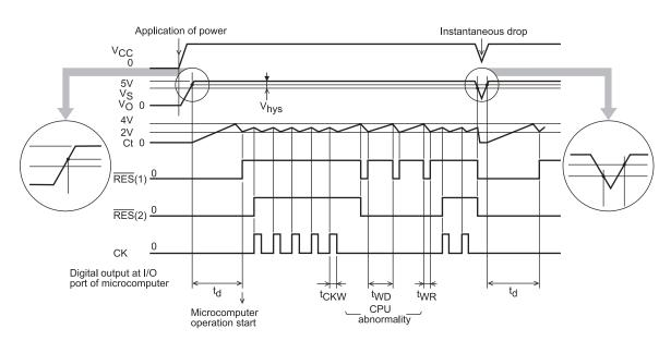
Note : Edge-triggered at the point indicated by the arrow of C<sub>K</sub> signal.
