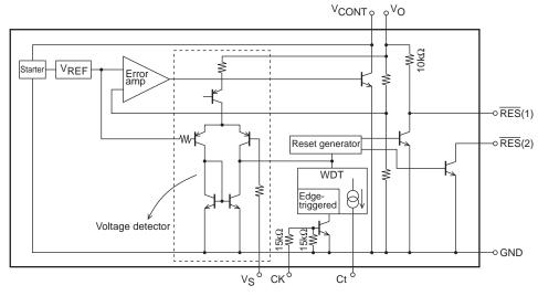
\*  $\overline{RES}(1)$  : Contains a pull-up resistor of 10k $\Omega$ .  $\overline{RES}(2)$  : Open collector
