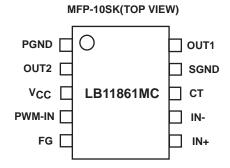
V<sub>CC</sub>: Common power supply for motor and control systems PGND: Motor system GND SGND: Control system GND
