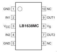
Note: both ground pins must be grounded.
