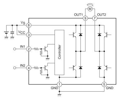
Note: When using the same power supply for  $V_S$  and  $V_{CC}$ , short the  $V_{CC}$  and  $V_S$  pins to each other or insert a capacitor in the  $V_{CC}$  line.
