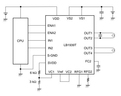
Channel 1 operates in constant voltage control mode: OUT outputs  $V_{DD} \times 3K/(3K + 6K) \times 1.95$ Channel 2 operates in constant current control mode: The RFG voltage is controlled so that Vref/4.5 = 0.2 V. \* : FC1 is left open.
