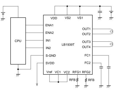
Constant current control mode: The RFG voltage is controlled so that Vref/4.5 = 0.2 V. Therefore, when RfB is 1  $\Omega$ , the circuit operates in constant current drive with lcoil = 0.2 V/1  $\Omega$  = 200 mA.
