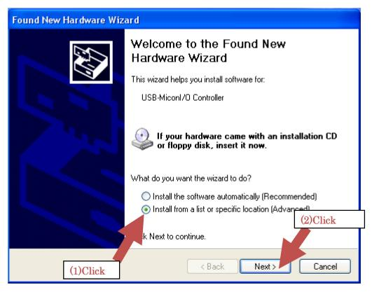
Figure 6. Driver Installation - Step 1
