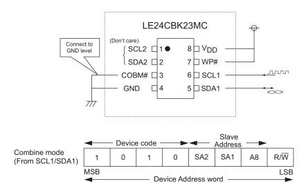
In combine mode, the slave address (SA2, SA1) is don't care, and any combination can be entered (SA2 = 1, SA1 = 1 or SA2 = 1, SA1 = 0 or SA2 = 0, SA1 = 1 or SA2 = 0, SA1 = 0).
