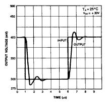
Figure 8. Voltage Follower Pulse Response (Small Signal)
