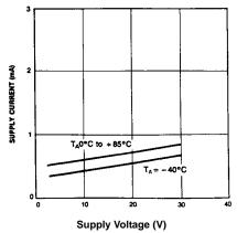
Figure 3. Supply Current vs Supply Voltage
