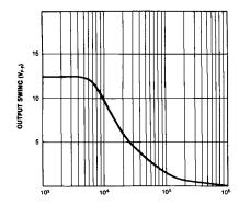
Figure 9. Large Signal Frequency Response
