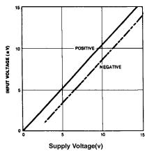
Figure 1. Input Voltage Range vs Supply Voltage
