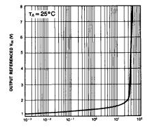
Figure 10. Output Characteristics vs Current Sourcing
