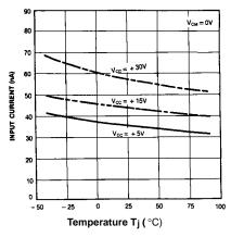
Figure 2. Input Current vs Temperature
