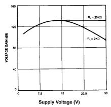
Figure 4. Voltage Gain vs Supply Voltage
