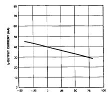
Figure 12. Current Limiting vs Temperature
