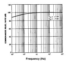
Figure 6. Common mode Rejection Ratio
