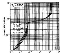
Figure 11. Output Characteristics vs Current Sinking
