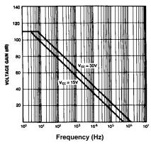
Figure 5. Open Loop Frequency Response
