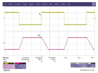
Figure 12. Inverting Large Signal Step Response
