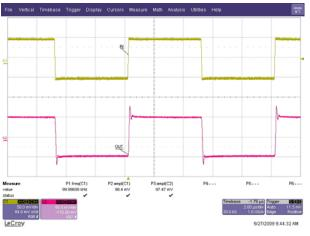
Figure 11. Non–Inverting Small Signal Step Response
