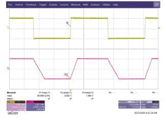
Figure 10. Non–Inverting Large Signal Step Response
