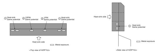
• Frame diagram (LV5680P) \*In the system power supply other than LV5680P, pin assignment may differ.
