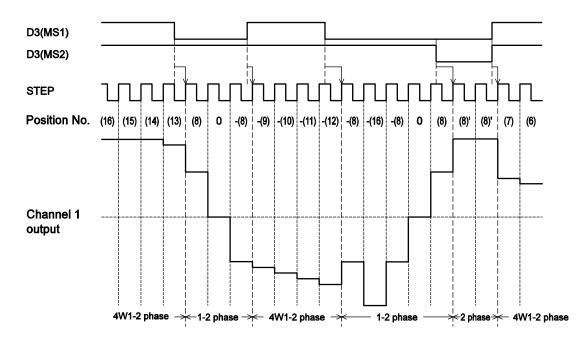
If the excitation mode is switched when power is applied to the motor, the operation follows the sequence shown below. (CW mode)
