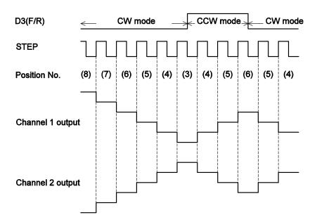
The IC internal D/A converter advances by 1 bits on the rising edge of the input step pulse.
