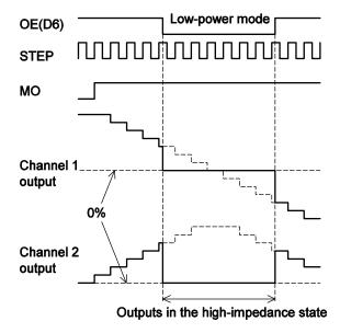
When the OE bit in the serial data, D6 (100, \*\*\*, D6, \*), is set to 0, the output is turned off and set to the high-impedance state at the rise of STB.
