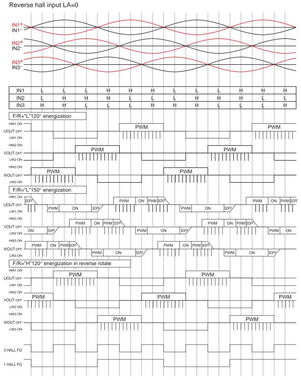
The energization is switched to  $120^{\circ}$  when 3 Hall FG frequency is 6.1Hz (TYP) or lower A direction of rotation is detected from Hall signal according to F/R pin input
