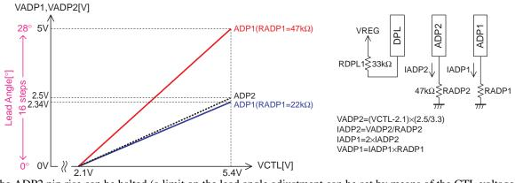
2. The ADP2 pin rise can be halted (a limit on the lead angle adjustment can be set by means of the CTL voltage) by setting DPL (pin 10).
