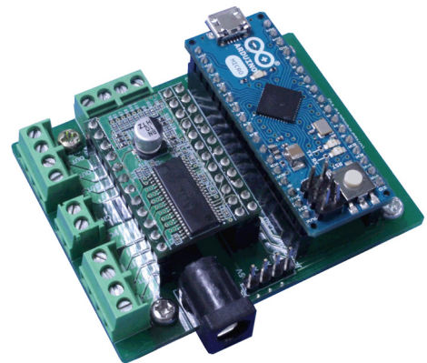
Figure 2. ONBB4AMGEVB Board with Arduino Micro and LV8702VSLDGEVB Board
