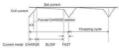
Charge mode continues until  $I_{COIL} \ge I_{REF}$ . After that the IC switches to SLOW DECAY mode and then switches to FAST DECAY mode for the last about 1 µs.
