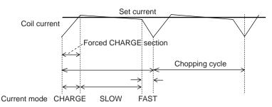
The IC switches to SLOW DECAY after Blanking section, and then switches to FAST DECAY mode for the last about 1µs.
