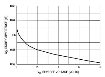
Figure 4. Diode Capacitance
