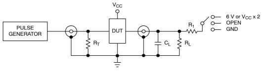
Figure 4. Test Circuit
