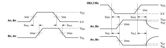
WAVEFORM 1 - PROPAGATION DELAYS  $t_R$  =  $t_F$  = 2.5 ns, 10% to 90%; f = 1 MHz;  $t_W$  = 500 ns WAVEFORM 2 - OUTPUT ENABLE AND DISABLE TIMES  $t_R$  =  $t_F$  = 2.5 ns, 10% to 90%; f = 1 MHz;  $t_W$  = 500 ns
