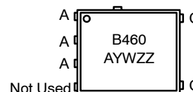
SO-8 FLAT LEAD CASE 488AA STYLE 2
