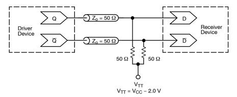
Figure 3. Typical Termination for Output Driver and Device Evaluation (See Application Note <u>AND8020/D</u> – Termination of ECL Logic Devices.)
