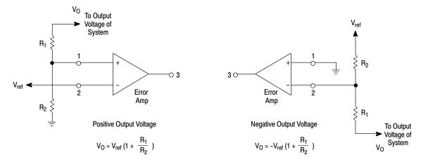
Figure 15. Error Amplifier Sensing Techniques
