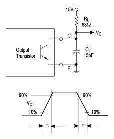
Figure 13. Common–Emitter Configuration and Waveform
