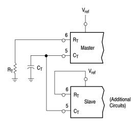
Figure 18. Slaving Two or More Control Circuits
