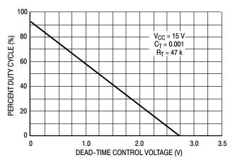
Figure 6. Percent Duty Cycle versus Dead-Time Control Voltage
