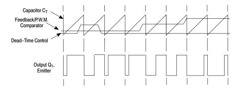
Figure 2. Timing Diagram
