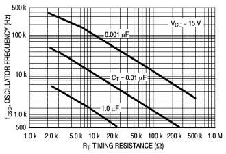
Figure 3. Oscillator Frequency versus Timing Resistance
