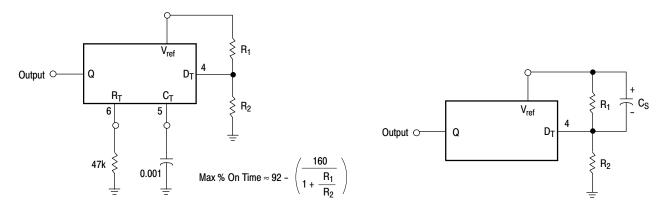
Figure 16. Deadtime Control Circuit
