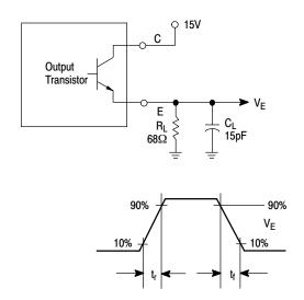
Figure 14. Emitter-Follower Configuration and Waveform
