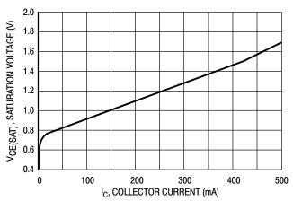
Figure 8. Common-Emitter Configuration
