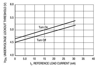
Figure 10. Undervoltage Lockout Thresholds versus Reference Load Current
