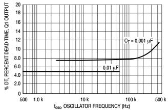
Figure 5. Percent Deadtime versus Oscillator Frequency
