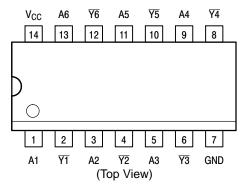
Figure 2. Pinout: 14-Lead Packages
