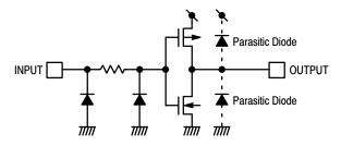
Figure 5. Input Equivalent Circuit
