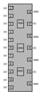
Figure 2. Pin Configuration
