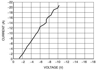
Figure 9. Negative TLP I-V Curve
