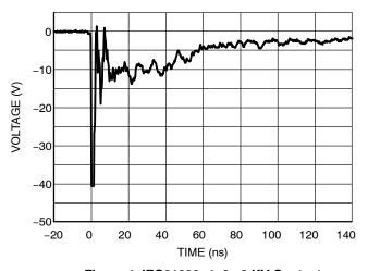
Figure 4. IEC61000-4-2 -8 KV Contact Clamping Voltage
