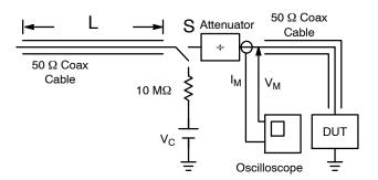
Figure 10. Simplified Schematic of a Typical TLP System
