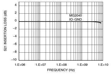
Figure 13. MG2040 Insertion Loss
