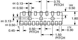
NOTE: CENTER PADS OPTIONAL DIMENSION: MILLIMETERS
