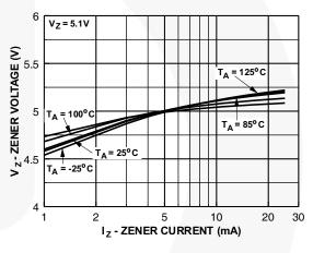
Figure 4. 5.1 Zener Voltage vs. Temperature
