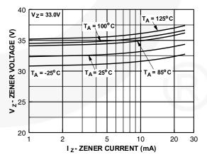
Figure 6. 33 Zener Voltage vs. Zener Temperature
