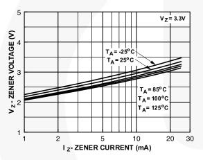
Figure 3. 3.3 Zener Voltage vs. Temperature
