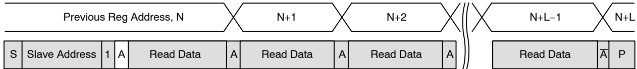
Figure 19. Sequential READ, Start from Current Location
