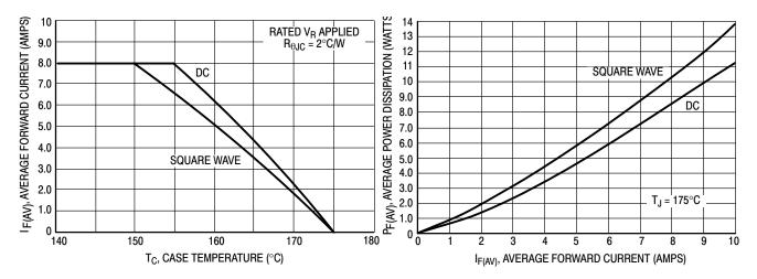
Figure 3. Current Derating, Case, Per Leg
