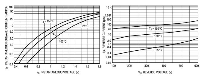
Figure 1. Typical Forward Voltage, Per Leg
