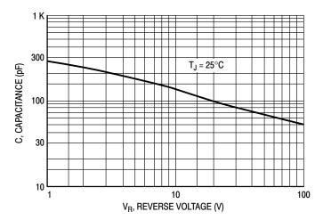
Figure 6. Typical Capacitance, Per Leg
