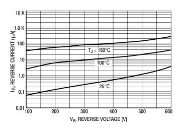
Figure 2. Typical Reverse Current, Per Leg\*
