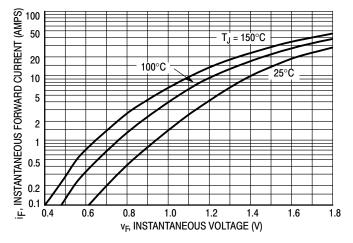
Figure 1. Typical Forward Voltage, Per Leg
