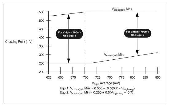
Figure 16. V<sub>cross</sub> Range Clarification (Note 40)
