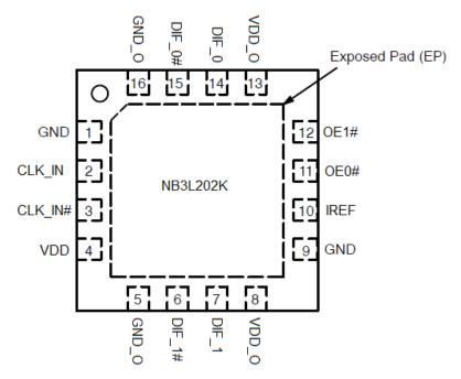
Figure 2. 16-Pin QFN Pinout (Top View)
