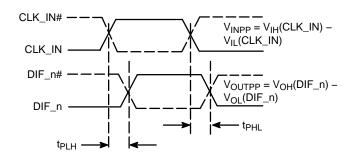
Figure 9. AC Reference Measurement
