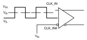
Figure 4. Differential Input Driven Single–Ended
