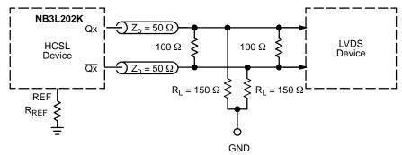
Figure 12. HCSL Interface Termination to LVDS
