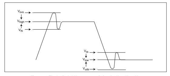
Figure 14. Single–Ended Measurement Points for  $V_{\rm ovs},\,V_{\rm uds},\,V_{\rm rb}$
