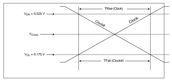
Figure 13. Single-Ended Measurement Points for Trise, Tfall
