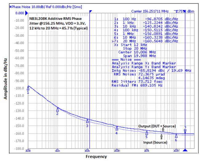
Figure 3. Typical Phase Noise Plot at f<sub>carrier</sub> = 156.25 MHz at an Operating Voltage of 3.3 V, Room Temperature
