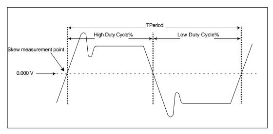
Figure 15. Differential (CLOCK - CLOCK#) Measurement Points (Tperiod, Duty Cycle)
