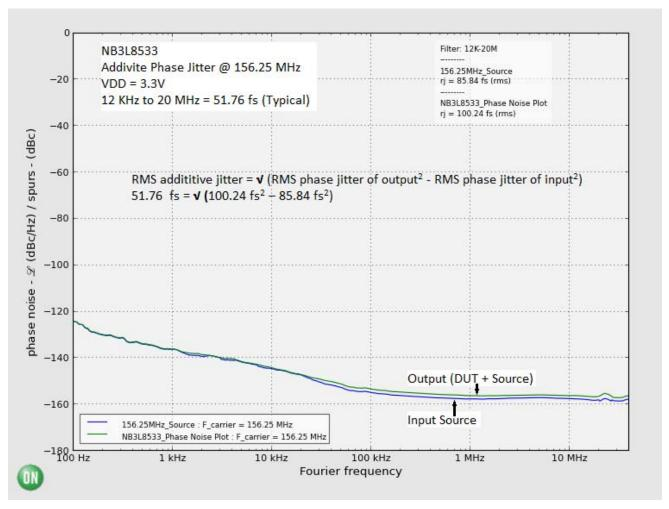
Figure 3. Typical Phase Noise Plot at f<sub>carrier</sub> = 156.25 MHz at an Operating Voltage of 3.3 V, Room Temperature
