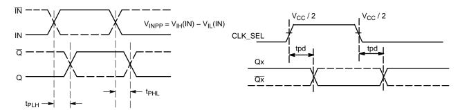
Figure 6. AC Reference Measurement
