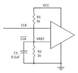
Figure 8. Differential Input Driven Single-ended
