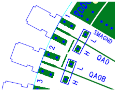
Figure 4. LVPECL Output Configuration
