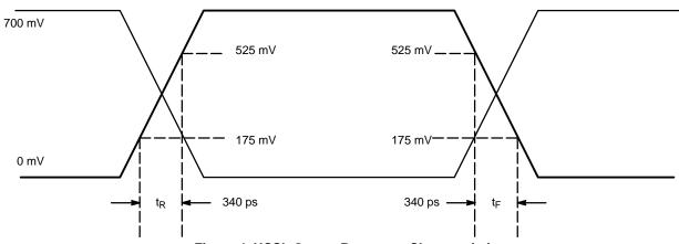
Figure 4. HCSL Output Parameter Characteristics
