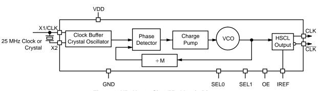
Figure 1. NB3N3002 Simplified Logic Diagram
