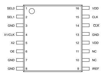
Figure 2. Pin Configuration (Top View)
