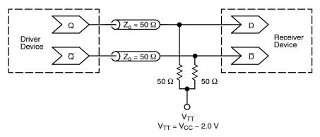
Figure 5. Typical Termination for Output Driver and Device Evaluation (See Application Note <u>AND8020/D</u> – Termination of ECL Logic Devices.)
