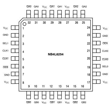
Figure 2. 32-Lead LQFP Pinout (Top View)
