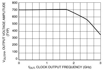
Figure 4. Output Voltage Amplitude (V<sub>OUTPP</sub>) versus Clock Output Frequency at Ambient Temperature (Typical)
