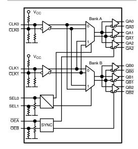
Figure 1. Functional Block Diagram
