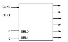
Figure 7. 1:6 Clock Fanout Buffer
