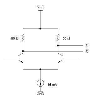
Figure 17. CML Output Structure
