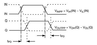
Figure 9. AC Reference Measurement
