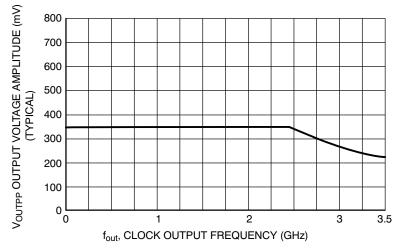
Figure 15. Output Voltage Amplitude (V<sub>OUTPP</sub>) versus Output Frequency at Ambient Temperature (Typical)
