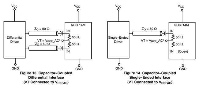
\*V\_{REFAC} bypassed to ground with a 0.01  $\mu\text{F}$  capacitor
