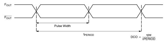
Figure 18. Output Duty Cycle
