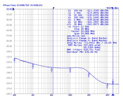
Figure 3. Typical Phase Noise Plot at 106.25 MHz
