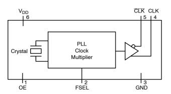
Figure 1. Simplified Logic Diagram
