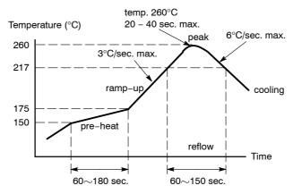
Figure 6. Recommended Reflow Soldering Profile
