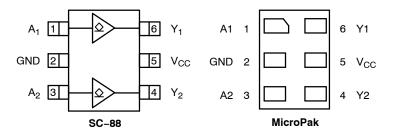
Figure 1. Pinout Diagrams (Top Views)
