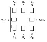
Figure 4. Pad Assignments for MicroPak (Top Through View)
