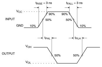
Figure 7. AC Waveforms
