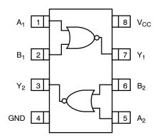
Figure 2. Pin Assignment for US8 (Top View)
