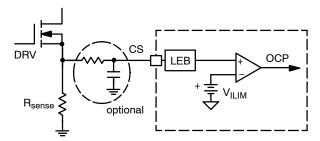
Figure 28. OCP Circuitry with Optional External RC Filter
