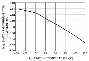
Figure 22. Switching Current Consumption vs. Junction Temperature
