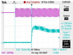
Figure 37. Start up Characteristic with 36.9 V, 350 mA Load
