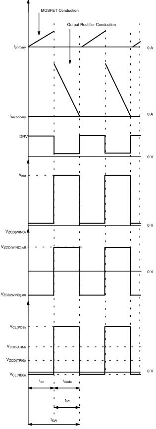
Figure 26. Ideal CrM Waveforms with ZCD Winding
