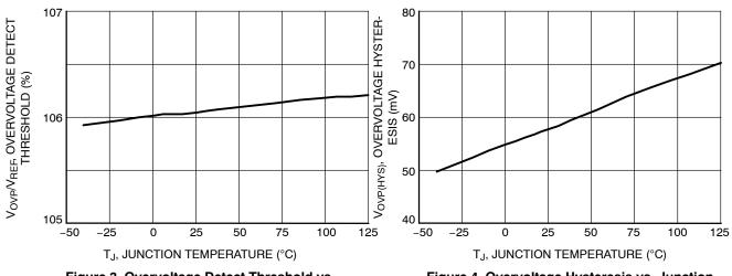
Figure 3. Overvoltage Detect Threshold vs. Junction Temperature
