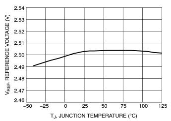
Figure 7. Reference Voltage vs. Junction Temperature
