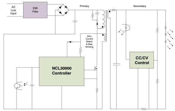
Figure 23. Simplified Block Diagram
