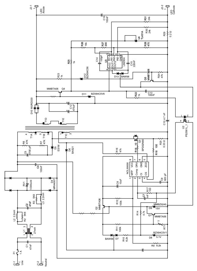
Figure 30. Wide Input Main, 4-15 LED 350 mA Load Schematic
