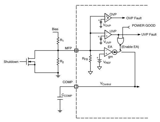
Figure 29. Multi-Function Pin Operation
