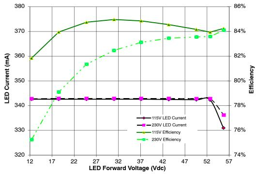
Figure 33. LED Current and Efficiency at 115 and 230 Vac
