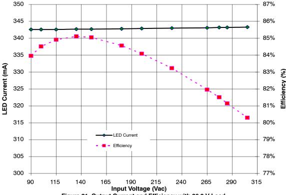
Figure 31. Output Current and Efficiency with 36.9 V Load
