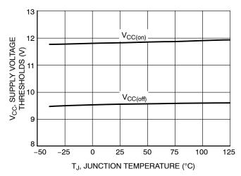
Figure 20. Supply Voltage Thresholds vs. Junction Temperature
