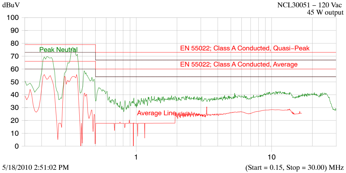
Figure 17. Conducted EMI Spectrum at 1 A with V_f = 45 V (Red = average)
