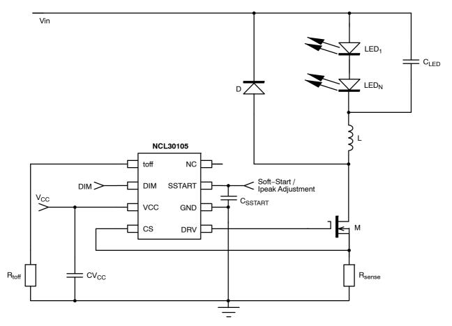
Figure 1. Typical Application Diagram
