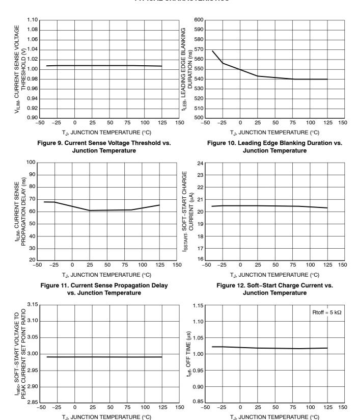
Figure 13. Soft-Start Voltage to Peak Current Set Point Ratio vs. Junction Temperature
