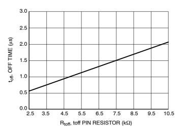
Figure 21. Zoomed In Off Time vs. toff Pin Resistor
