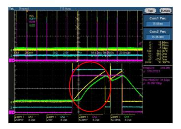
Figure 31. Minimum Dimming Duty Cycle
