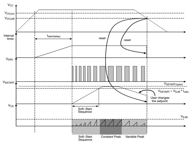
Figure 22. A Typical Startup Sequence
