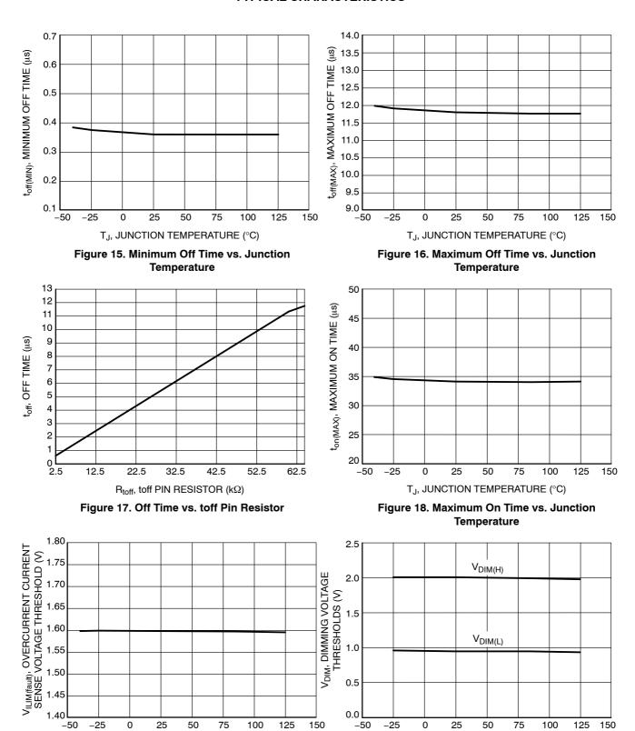
Figure 19. Overcurrent Current Sense Voltage
