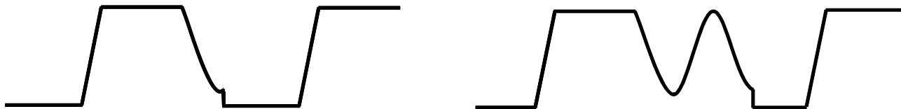
Figure 7. Quasi-resonant Mode in Low Line (left), Turn on at Valley 2 when in High Line (right)
