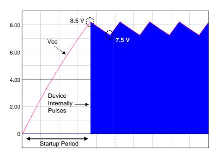
Figure 16. The Charge/Discharge Cycle Over a 10 µF V<sub>CC</sub> Capacitor
