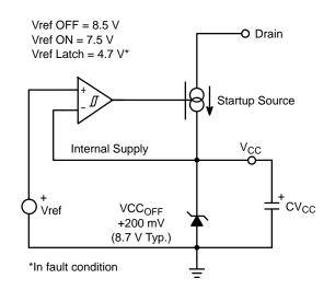
Figure 15. The Current Source Regulates V<sub>CC</sub> by Introducing a Ripple
