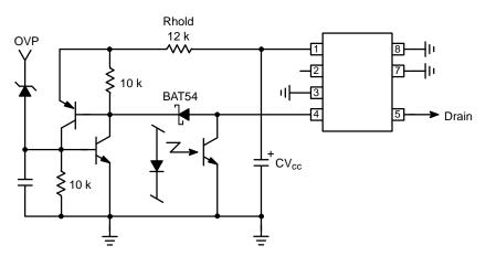
Figure 26. Two Bipolars Ensure a Total Latch-Off of the SMPS in Presence of an OVP
