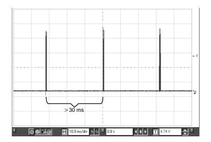
Figure 21. The burst frequency becomes so low that it is difficult to keep an adequate level on the auxiliary  $V_{CC}$ ...
