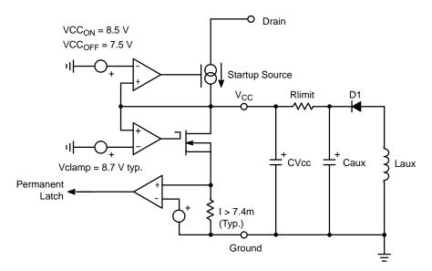
Figure 20. A more detailed view of the NCP101X offers better insight on how to properly wire an auxiliary winding.
