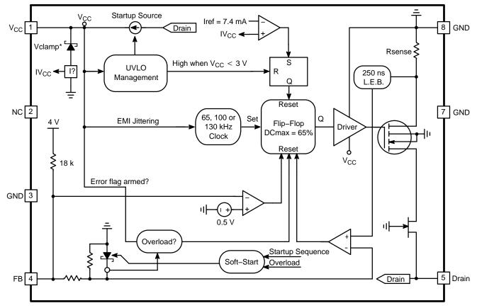
\*Vclamp = VCC<sub>OFF</sub> + 200 mV (8.7 V Typical)
