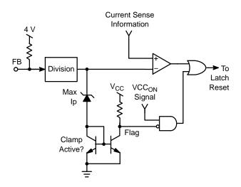
Figure 17. Simplified NCP101X Short–Circuit Detection Circuitry
