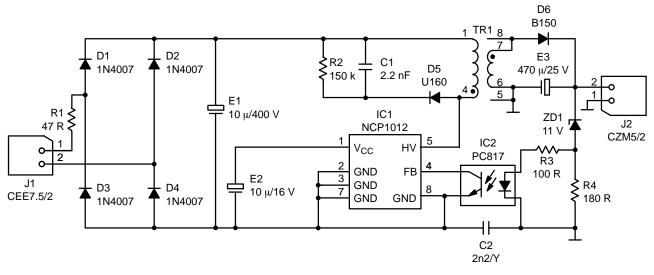
Figure 30. An NCP1012–Based Flyback Converter Delivering 6.5 W
