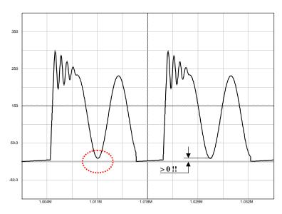
Figure 28. The Drain–Source Wave Shall Always be Positive . . .
