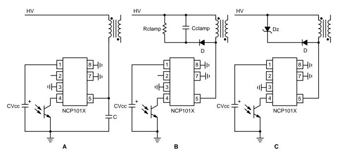
Figure 29. Different Options to Clamp the Leakage Spike
