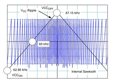
Figure 23. The V<sub>CC</sub> ripple is used to introduce a frequency jittering on the internal oscillator sawtooth. Here, a 65 kHz version was selected.
