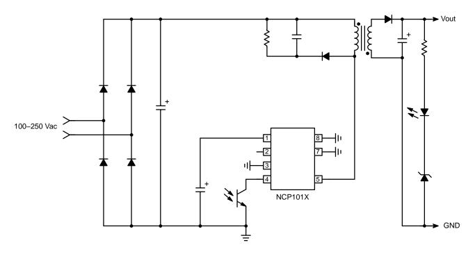
Figure 1. Typical Application Example
