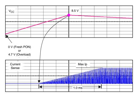
Figure 24. Soft-Start is activated during a startup sequence or an OCP condition.
