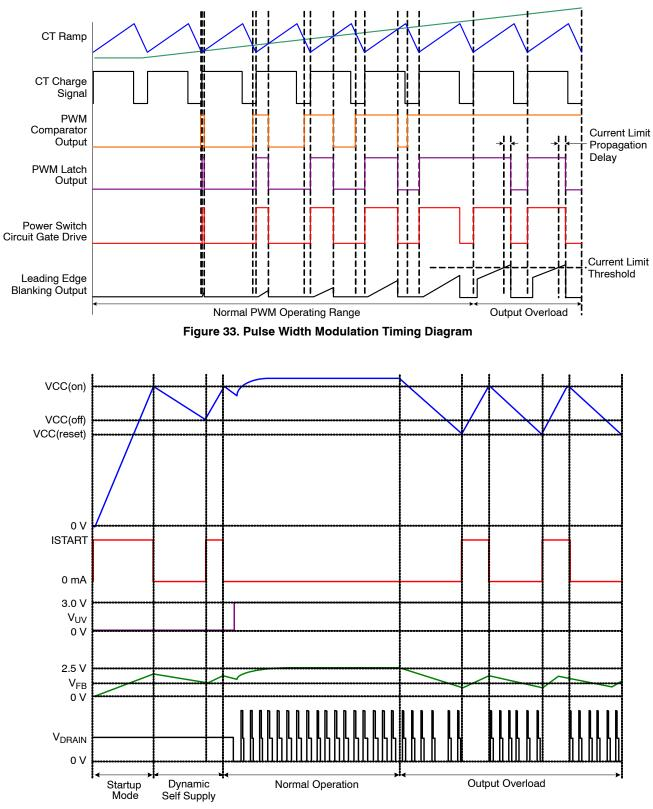
Figure 34. Auxiliary Winding Operation with Output Overload Timing Diagram
