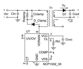
Figure 45. Passive RCD Clamp Network
