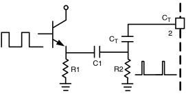
Figure 40. External Frequency Synchronization Circuit
