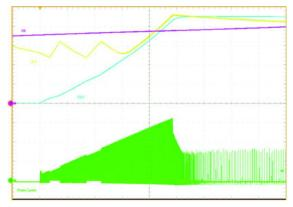
Figure 6. Soft–Start, R<sub>CL</sub> open, Output No Load 1 V<sub>CC</sub> 3.0 V/div DC, 2 V<sub>OUT</sub> 3.0 V/div DC, 3 VIN 10.0 V/div DC, 4 I<sub>PRI</sub> 100 mA/div DC,  $T = 500 \ \mu$ s/div
