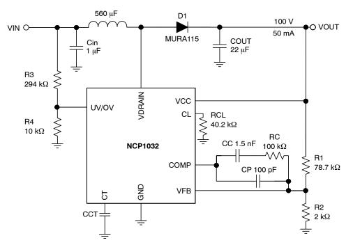
Figure 51. Typical Application Circuit Boost Circuit Configuration
