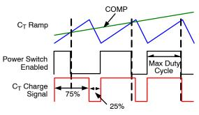
Figure 39. Auxiliary Winding Operation with Output Overload Timing Diagram
