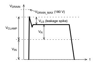
Figure 44. Power Switch Waveforms with Clamping
