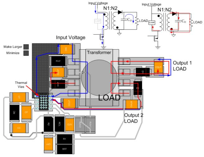
Figure 48. Recommended PCB Layout
