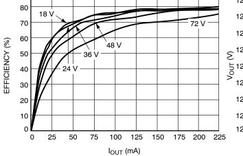
Figure 3. Efficiency vs. I<sub>OUT</sub> at V<sub>IN</sub> = 24, 36, 48 and 72 V, T1 = CoilCraft B0226–EL
