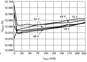
Figure 4. V<sub>CC</sub> Pin Load Regulation at V<sub>IN</sub> = 24, 36, 48 and 72 V
