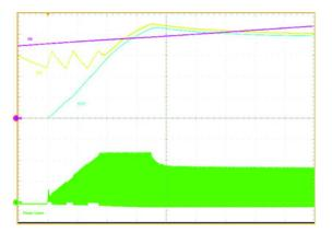
$\begin{array}{l} \mbox{Figure 7. Soft-Start, R_{CL} = 32 \ k\Omega \ (C_{LIM} = 250 \ mA), \ Output \ Load = 240 \ \Omega \ (I_{OUT} = 50 \ mA), \\ 1 \ V_{CC} \ 3.0 \ V/div \ DC, \ 2 \ V_{OUT} \ 3.0 \ V/div \ DC, \ 3 \ V_{IN} \\ 10.0 \ V/div \ DC, \ 4 \ I_{PRI} \ 100 \ mA/div \ DC, \\ T = 1.0 \ ms/div \end{array}$
