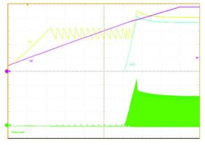
Figure 5. Startup Sequence, R<sub>CL</sub> Open, Output Load = 80  $\Omega$  (I<sub>OUT</sub> = 150 mA), 1 V<sub>CC</sub> 3.0 V/ div DC, 2 V<sub>OUT</sub> 3.0 V/div DC, 3 V<sub>IN</sub> 10.0 V/ div DC, 4 I<sub>PRI</sub> 100 mA/div DC, T = 20 ms/div
