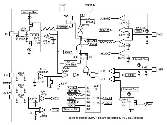
Figure 2. NCP1032 Simplified Block Diagram
