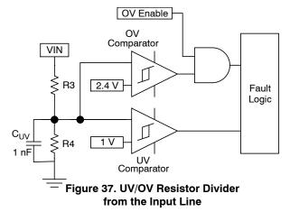
The resistive network impedance must not be too high to keep good voltage accuracy and not too low to minimize power losses. A 200 k $\Omega$  to 1.2 M $\Omega$  range is recommended for the high side resistor R3. If the designer wanted to set the undervoltage threshold to 32 V, the resistor divider should be designed according to the following equation:
