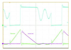
Figure 8. Discontinuous Conduction Mode (DCM),  $I_{OUT}$  = 150 mA, 2 V<sub>DRAIN</sub> 20 V/div DC, 3 I<sub>SEC</sub> 30 mA/div DC, 4 I<sub>PRI</sub> 100 mA/div, DC, T = 500 ns/div
