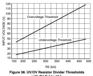
with R4 Set to 10 k The UV/OV pin can also be used to implement a remote
