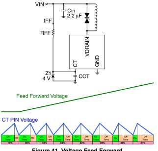
Figure 41. Voltage Feed Forward
