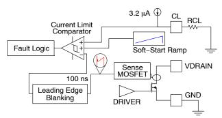
Figure 42. Current Limit Threshold and **Propagation Delay**
