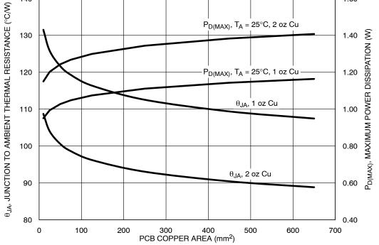
Figure 39.  $\theta_{JA}$  and P<sub>D (MAX)</sub> vs. Copper Area (CSP4)
