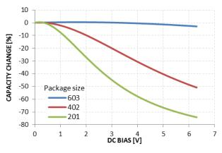
Figure 38. Capacity vs DC Bias Voltage
