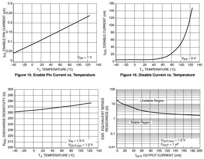
Figure 17. Discharge Resistivity vs. Temperature
