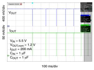
Figure 35. Overheating Protection – TSD
