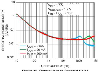
Figure 19. Output Voltage Spectral Noise Density vs. Frequency
