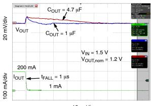
$\begin{array}{l} 10 \ \mu \text{s/div} \\ \text{Figure 32. Load Transient Response,} \\ I_{OUT} = 1 \ \text{mA to 200 mA} \end{array}$
