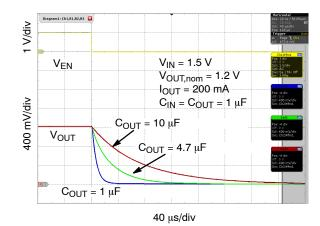
Figure 37. Enable Turn-off Response, Various Output Capacitors
