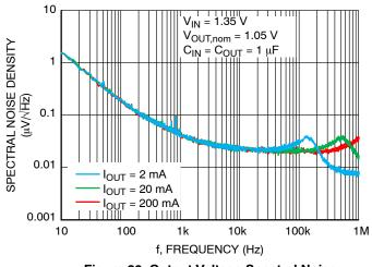
Figure 20. Output Voltage Spectral Noise Density vs. Frequency
