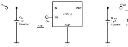
**Figure 1. Typical Application Schematics**
