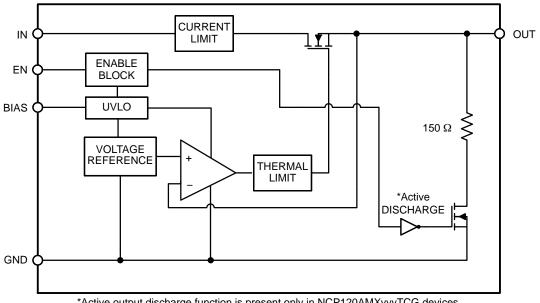
\*Active output discharge function is present only in NCP120AMXyyyTCG devices. yyy denotes the particular output voltage option.
