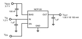
Figure 1. Typical Application Schematics
