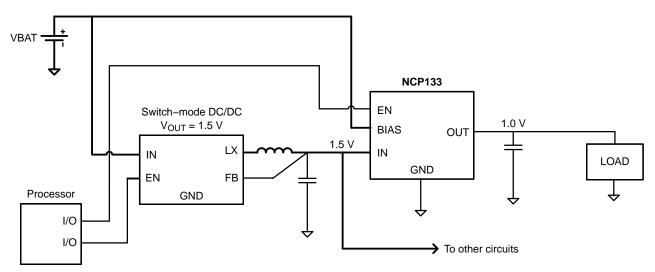
Figure 12. Typical Application: Low-Voltage DC/DC Post-Regulator with ON/OFF Functionality
