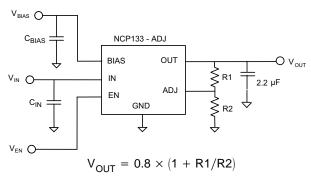
Figure 13. Typical Application Schematics
