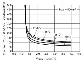
Figure 6.  $V_{IN}$  Dropout Voltage vs. ( $V_{BIAS}$  –  $V_{OUT}$ ) and Temperature  $T_J$
