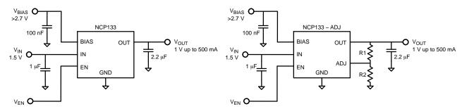
**Figure 1. Typical Application Schematics**
